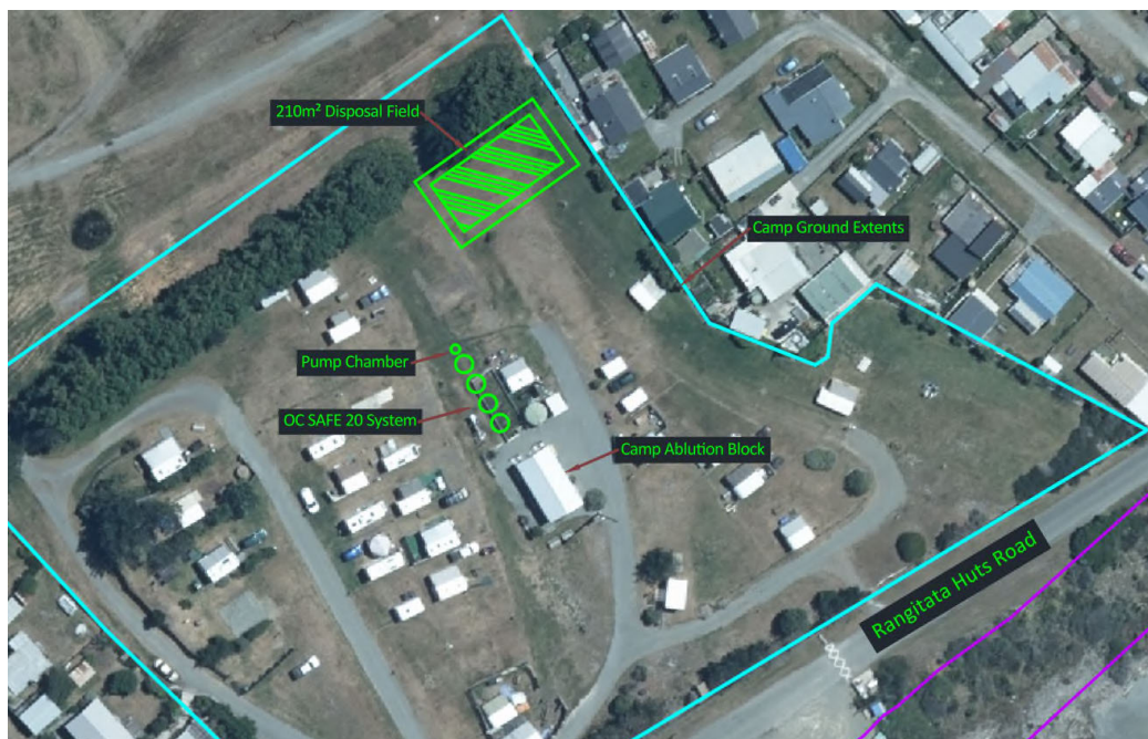
Figure 3: Campground Onsite Treatment System and Disposal Field
