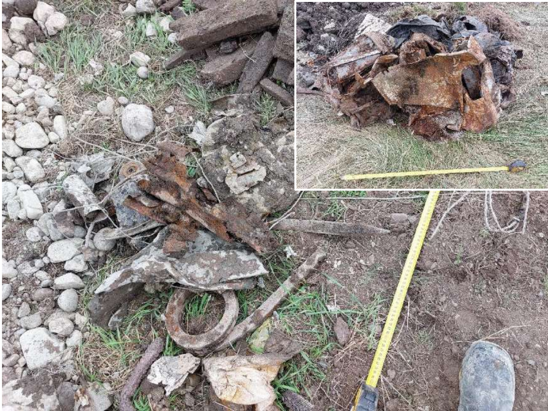
Photograph 21: Scrap metal separated from TP103 arisings. Inset shows some of the coarse fraction of scrap metal.
