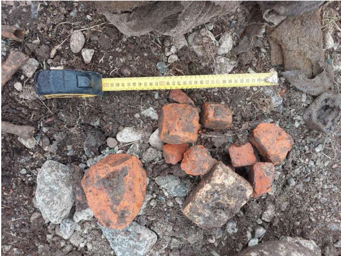
Photograph 29: Brick fragments separated from TP105 arisings.
