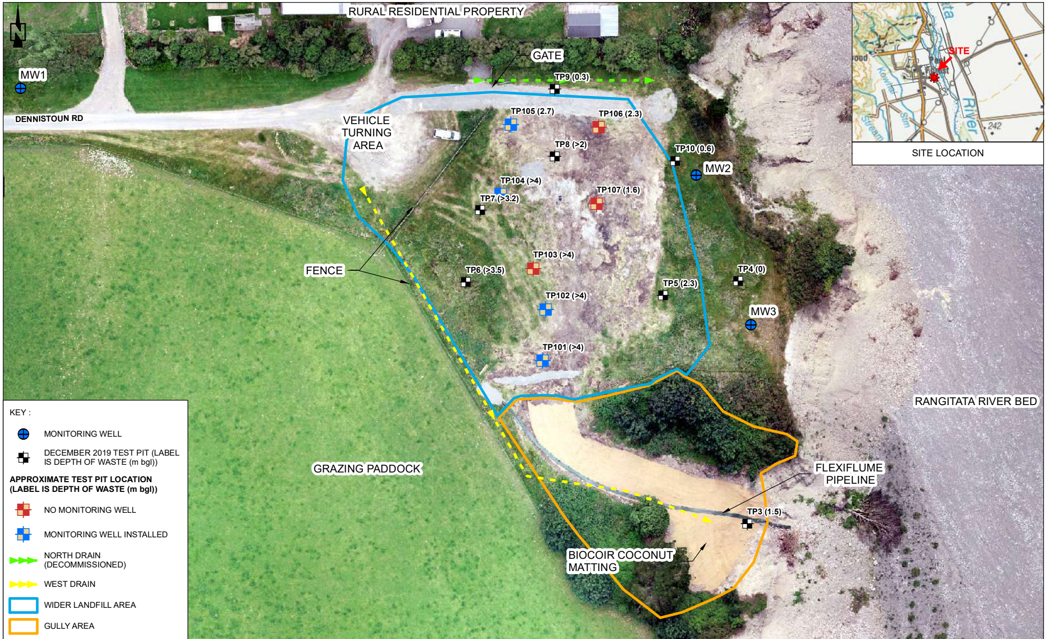
FIGURE 1 : PEEL FOREST LANDFILL FEATURES (SEPTEMBER 2022)
