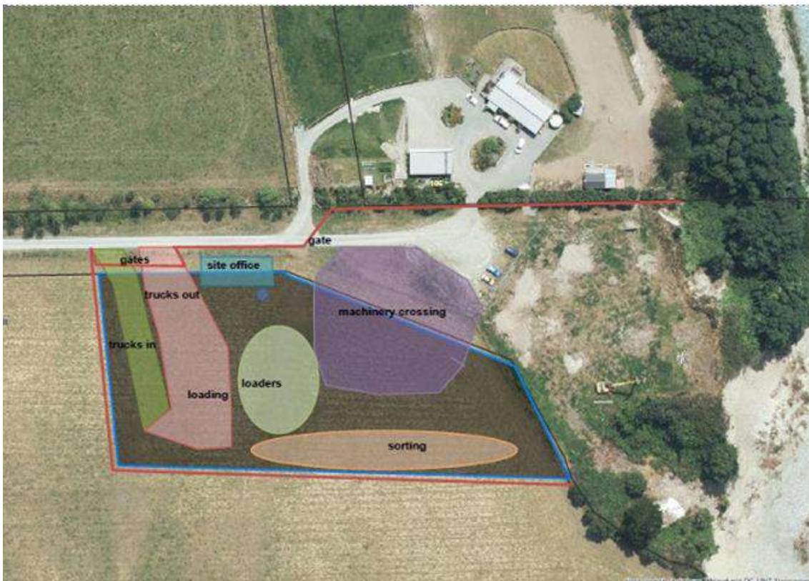
Figure 1: Indicative layout of contractor's yard (AEE Fig 3)
