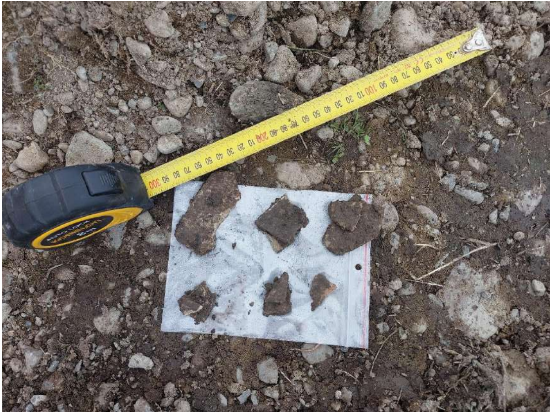
Photograph 27: ACM fragments separated from TP105 arisings.
