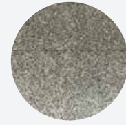
Exposed aggregate in situ concrete
