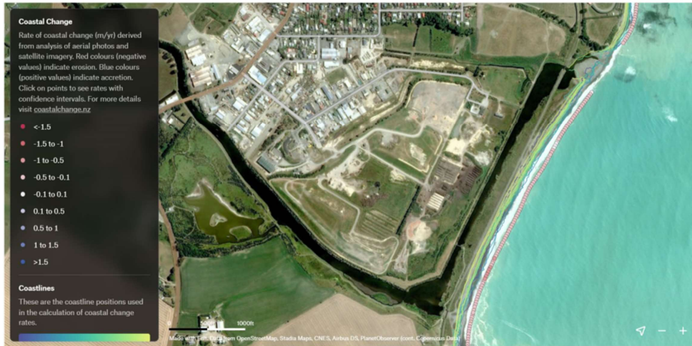
Figure 12. Rate of coastal change (m/yr) at Redruth Beach, where pink dots indicate erosion on the order of 0.5 to 1 m/year. Coloured lines show that the shoreline (based on the storm ridge since this is a gravel beach) has been receding landward since 1943 (Source: www.coastalchange.nz )
