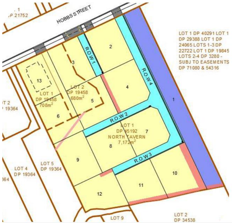
Figure 5 - Subdivision scheme plan for 18A Hobbs Street. Lot 1 (in blue) being a 10 m strip has been purchased by Foodstuffs from TDL.
